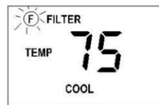
After changing or cleaning the system filter, press and hold the Filter hole for 3 seconds. The display will blink, and the counter will be reset to zero.
