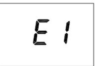
To correct this problem, replace the battery with 1 new AA alkaline battery, even if you have recently replaced them. Next, Move the battery out hold any key then place the battery again. You will need to reprogram your thermostat and confirm normal operation. If Error Mode returns, please call us for further information.
