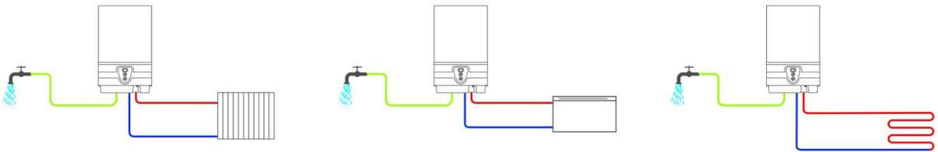
SISTEMAS POR: RADIADORES, FAN COILS, PISO RADIANTE Y ZOCALOS RADIANTES
