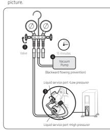
3 Open the valve of the low pressure side of manifold gauge anticlockwise.
