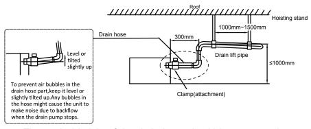
The vertical height of the drain hose should be 75mm or less so that it is unnecessary for the drain port to withstand additional force.
