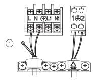
b) Wire routing of unified power supply:
