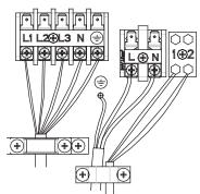
Power cord should be secured along with the right side plate and fixed to the hook with a wire clamp so as to avoid contacting the pipeline. The communication line between indoor and outdoor units should also be laid along with the right side plate but away from the power cord.
