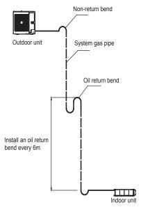
Dimensions for the making of oil return bend are as follows:
