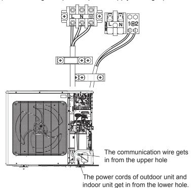
b) Wire routing of unified power supply for single phase.
