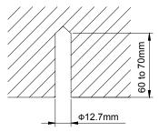
(2) Insert the anchor bolts into the drilled holes, and drive the pins completely into the anchor bolts with a hammer. See the following figure.
